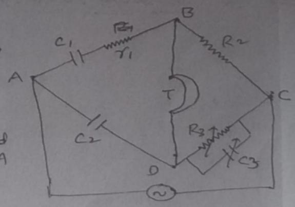
Here  $Z_1 = r_1 + \frac{1}{j\omega C_1}$ ,  $Z_2 = R_2$ ,  $Z_3 = \frac{1}{j\omega C_2}$ ,  $\frac{1}{Z_4} = \frac{1}{R_3} + \frac{1}{j\omega C_3} = \frac{1}{R_3} + j\omega C_3$
