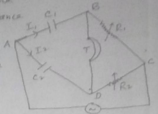
This bridge is suitable for comparing two capacitances in terms of two non inductive resistances. However, a perfect balance is not possible if there is some resistance of the capacitors, i.e. capacitors have some power factors. Here only quadrature components are balanced and in phase components are neglected assuming the capacitors to be perfect.
