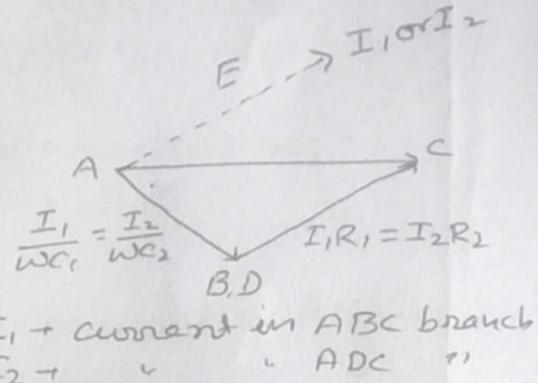
Since a part in a resistor  $R_d$  is in phase with the current,  $BC$  must be parallel to  $AE$ . At Balance  $D$  are at the same potential and so  $D$  also lies at  $B$  vector diagram, i.e. the current  $I_2$  is also along  $AE$ .
